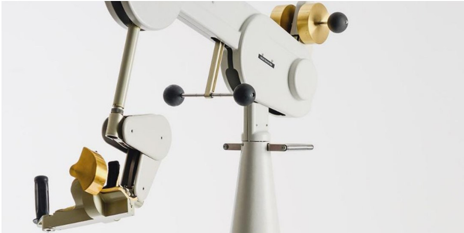
The body of the passive robotic arm called Track-Hold.
