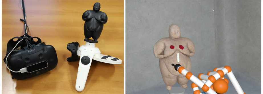
(Left) Photos of the hardware of the system: HTC Vive, LeapMotion, Vive Tracker, the 3D-printed support with the replica that hosts the controller for capacitive touch sensing. (Right) Example of a painting session.
