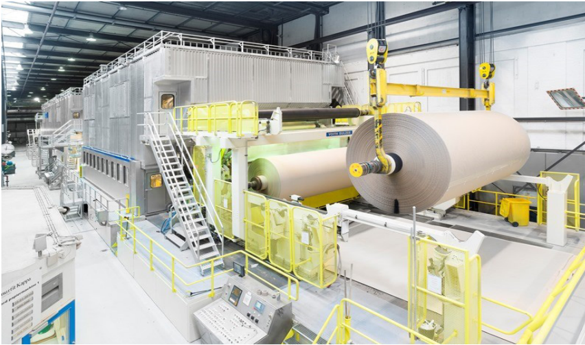
A paper machine with jumbo rolls in the foreground (from VOITH).
