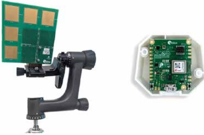
The XPLR-AOA kit with anchor node and tag.
