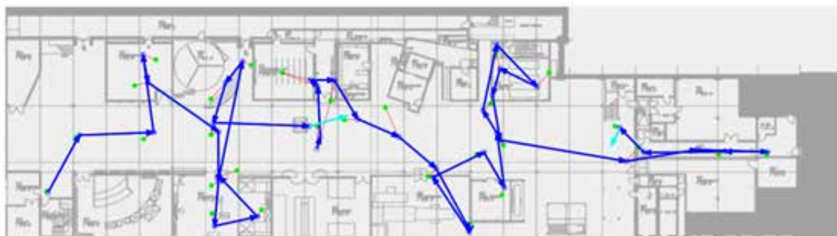
Path of the underground floor with errors for the thws team, winner of Track 1 (Markus Ebner, Steffen Kastner, Markus Bullmann, Toni Fetzer, Frank Deinzer) from the Technische Hochschule Würzburg-Schweinfurt. Green dots are reference points, small blue circles are estimated points, red lines show error size.
