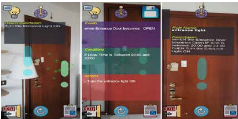
(Left) after configuring the trigger “Entrance door”, a recommendation is placed over the Entrance light; (centre) a schematic view of the rule currently in editing; (right) the “Explore environment” modality displays the created automations over the associated virtual objects.
