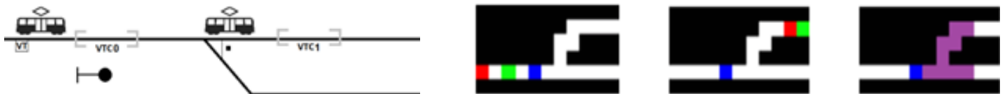
A scenario where one train is waiting to enter a junction area while another train is traversing it (leftmost) and (second from left to right) the initial configuration of the railway example, a final configuration in which both trains exit the junction from the same route, and the junction area emphasised in purple.
