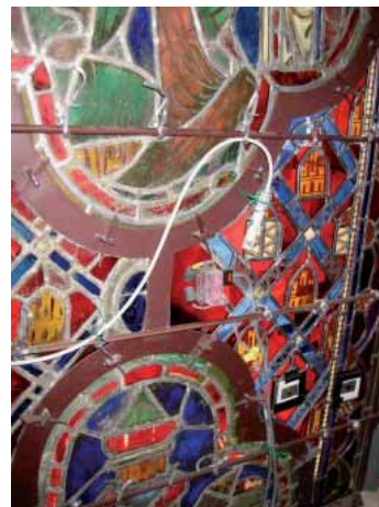
Fig. 3 Installazione del prototipo del dew sensor at the Sainte Chapelle (Paris-France).. Prototype of the dew sensor at the Sainte Chapelle (Paris-France).
