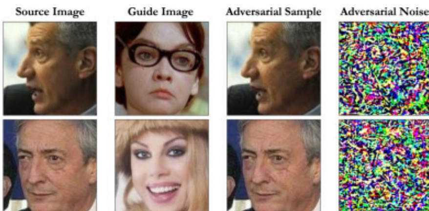
Adversarial examples for two different values of the threshold applied while solving the optimization problem. Top: \delta = 5.0 . Bottom: \delta = 10.0 .
